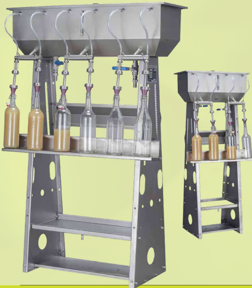
Cones are optionally available for seamless covering of different bottleneck diameters.
