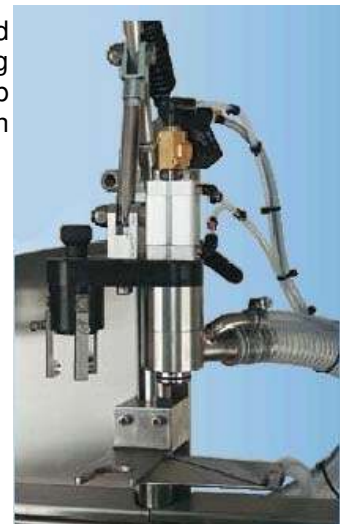
Bag retainer and hermetically closed filling head for no-drip operation
